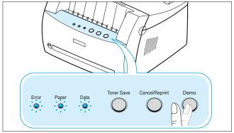
3 Your printer automatically picks up a sheet of paper from the tray and prints out a cleaning sheet with the dust or toner particles on it.
